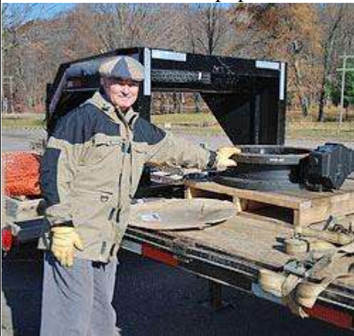
DNR limnologist Dick Lathrop pointed out the new flow valve to be installed in the withdrawal pipe.
