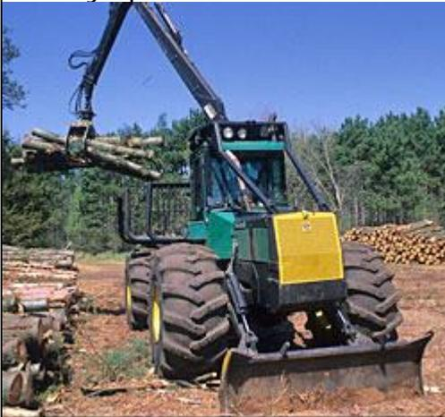
A forwarder carries felled logs clear of the ground from the stump to a roadside landing.
