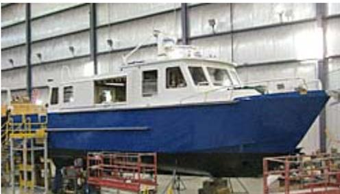
All major painting has been completed and the plastic paint booth has been taken down. In this photo you can see that in addition to being painted, the anchor on the bow and all of the equipment on the pilot
