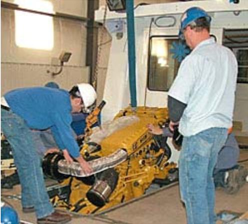
Brandon and Burger staff lowered the port engine into position through an aft deck soft patch. The starboard engine already is in place.
