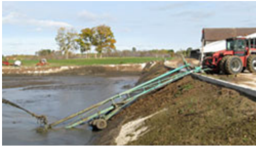
Typical agitation method used during liquid manure loading for land application to fields. DNR Photo
